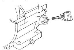
Figure 5. Engine Oil Dipstick
